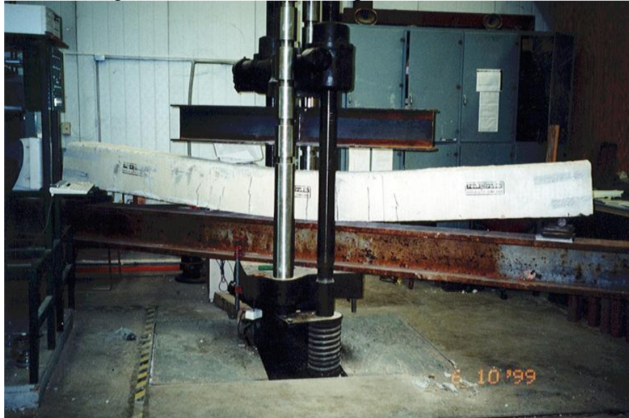
Figure 5a Typical Failure Mode for the Long-Span ICF Flat Lintel (4x12 specimen after excessive deflection and tensile steel yielding)
