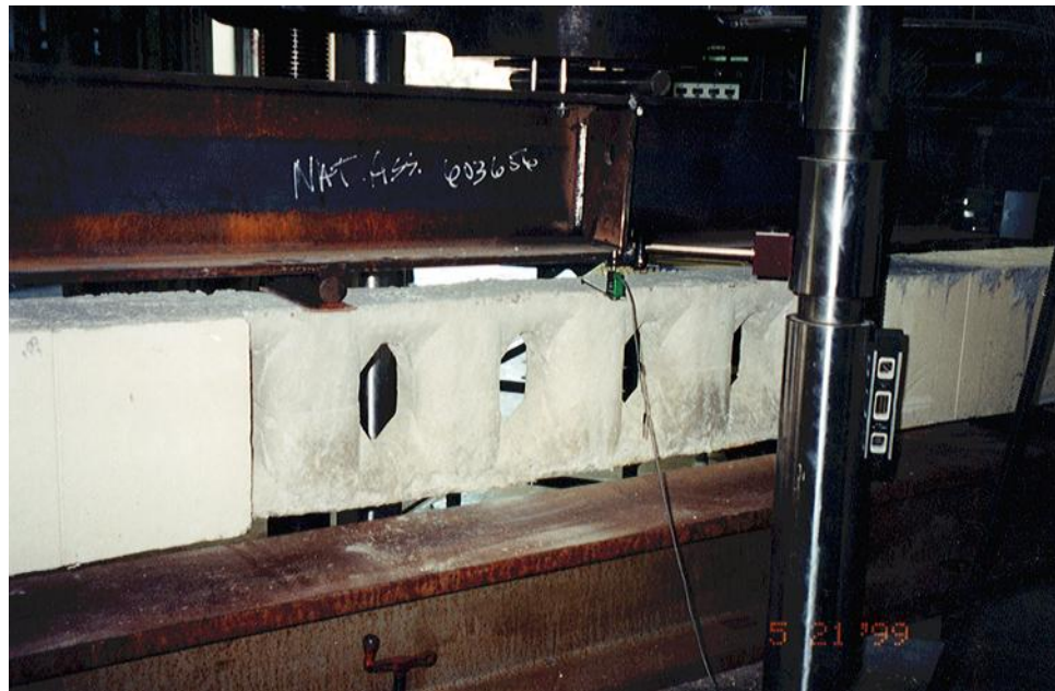
Figure 4 Steel I-Beam, Loading Points, and Deflectometer
