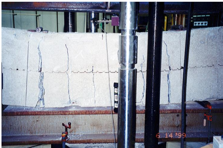
Figure 5b Typical Failure Mode for the Long-Span ICF Flat Lintel (4x24 specimen after excessive deflection and tensile steel yielding)
